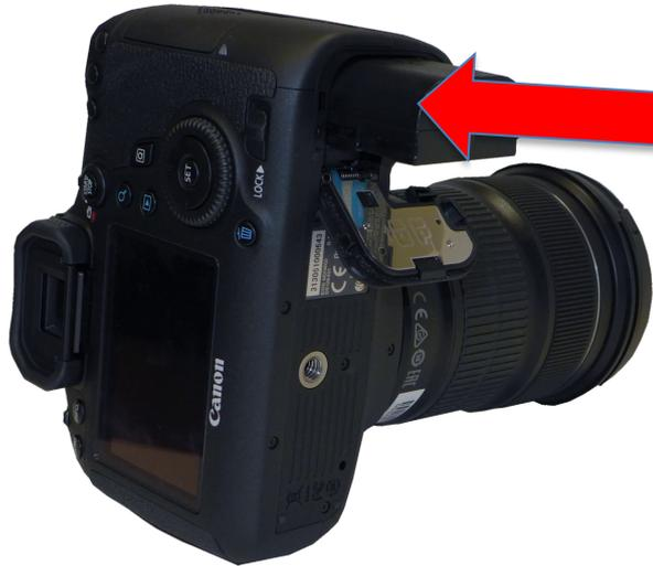
2. Insert the Media Card in the card slot of the camera.
