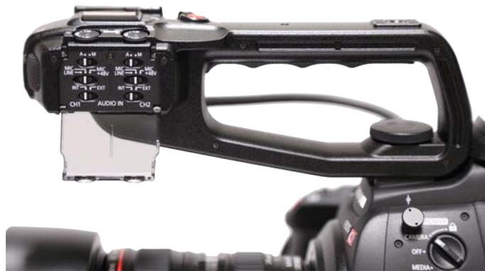
The camera handle can supply +48 V Phantom power to your microphone if it is needed.
