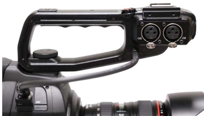
The handle can take two audio inputs by using XLR cable.
