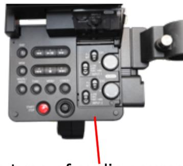
Set the type of audio source. (mic, line, mic with phantom power)
